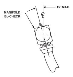
**Note:** Install El-Check so that arrow is in direction indicated. El-Check may be adjusted as shown to obtain a smooth radius in flexible discharge hose.
